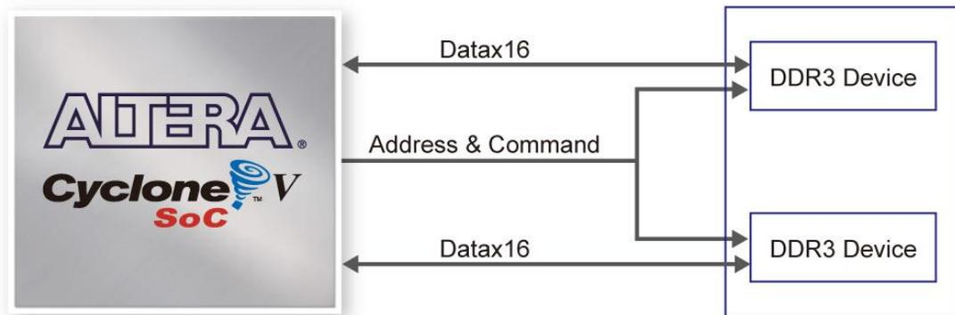
**Figure 3-26 Connections between FPGA and DDR3**
