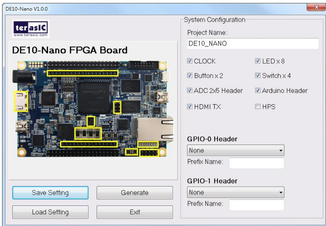
**Figure 4-2** The GUI of DE10-Nano System Builder
