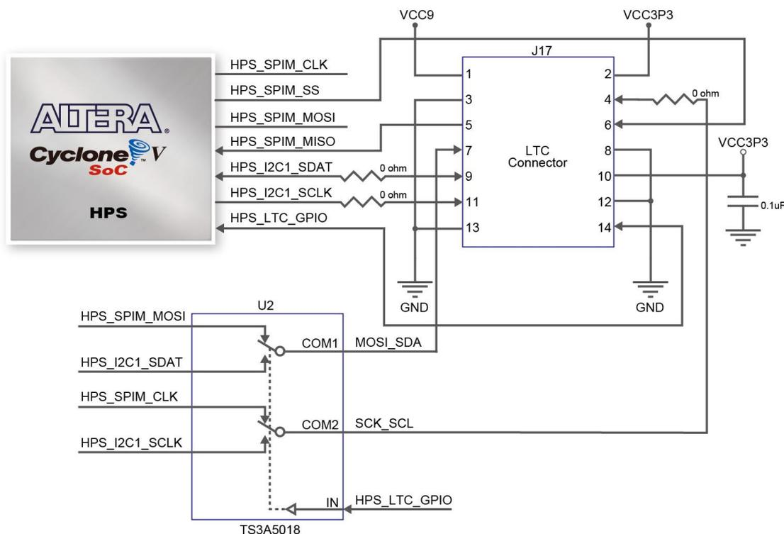
**Figure 3-30 Connections between the HPS and LTC connector**
