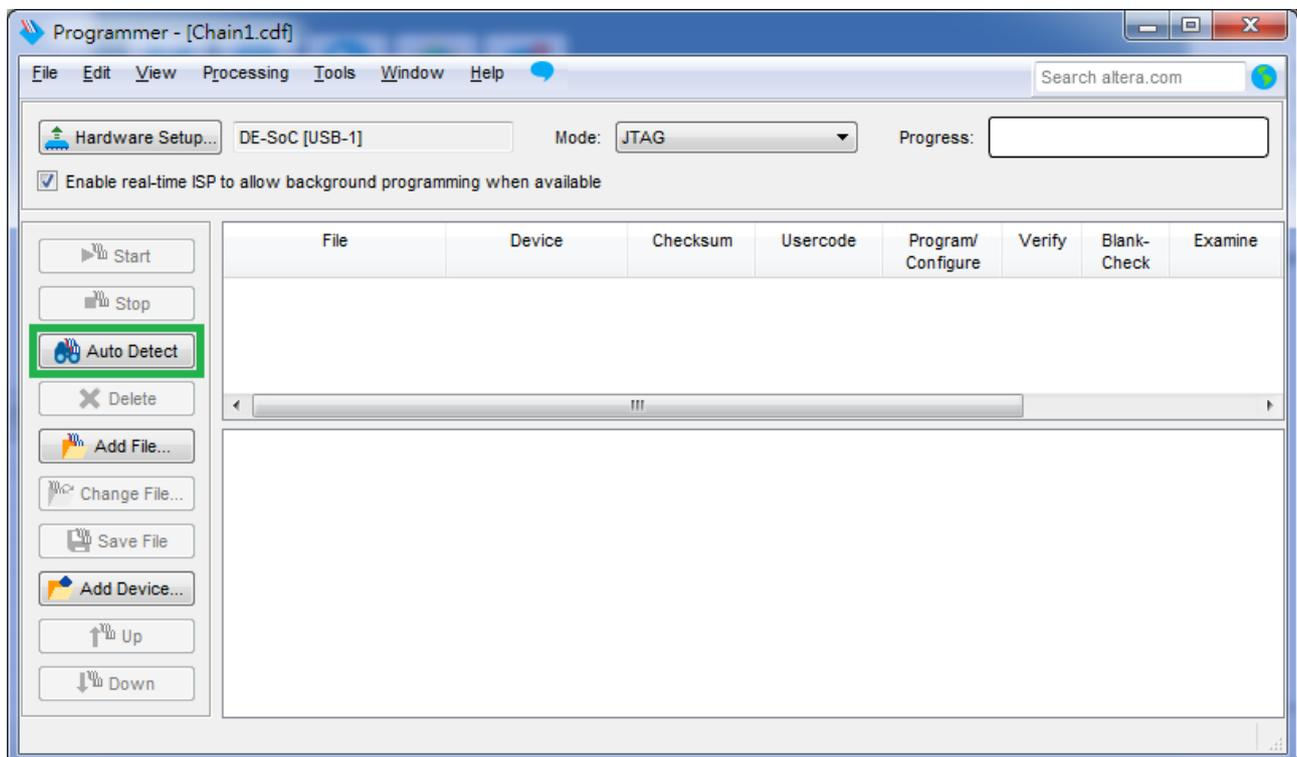
**Figure 3-5 Detect FPGA device in JTAG mode**
