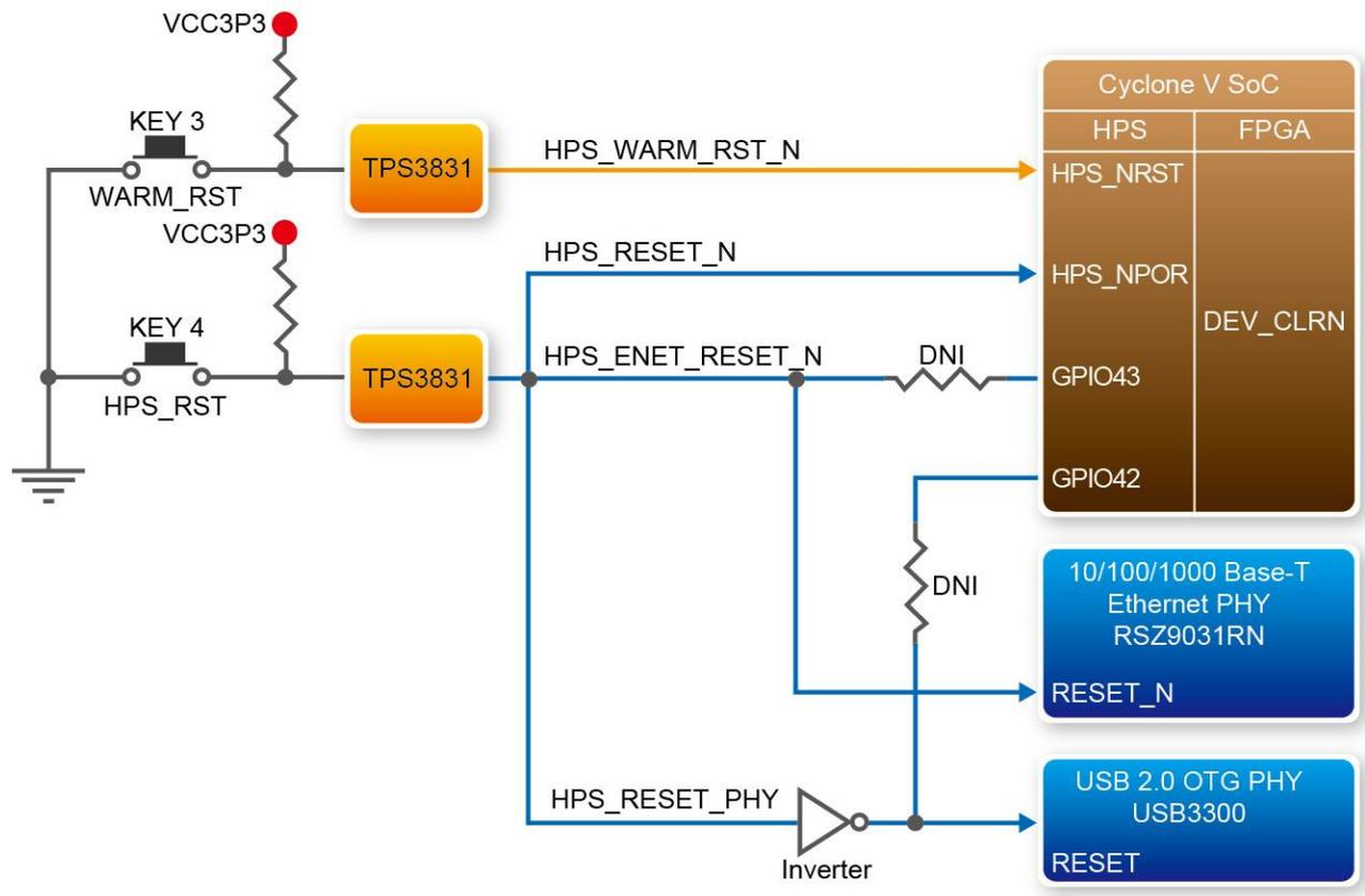
Figure 3-14 HPS reset tree on DE10-Nano board
