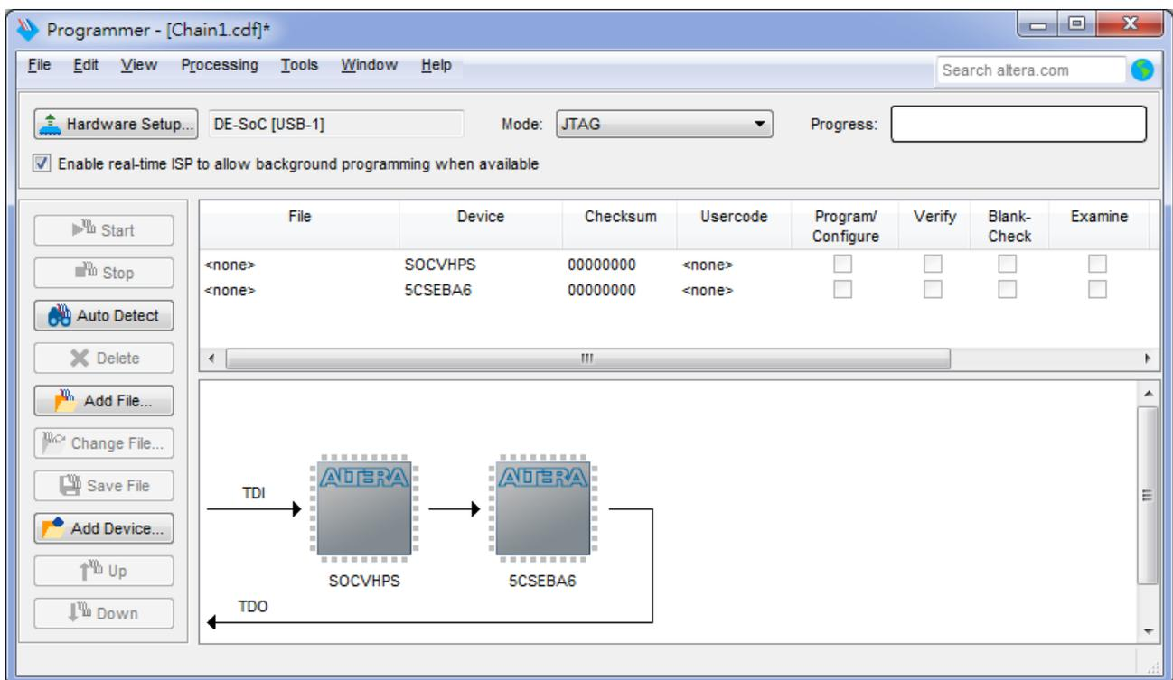
**Figure 3-7 FPGA and HPS detected in Quartus programmer**
