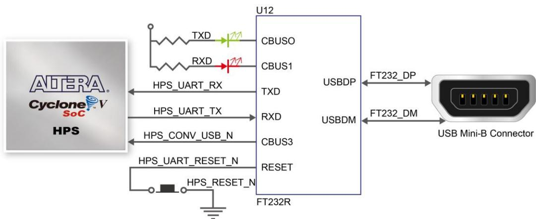
**Figure 3-25 Connections between the HPS and FT232R Chip**
