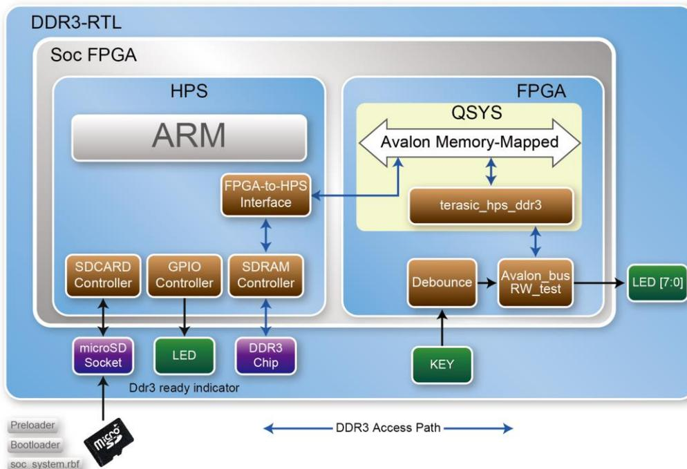
**Figure 5-14** Block Diagram of the DDR3\_RTL Demonstration
