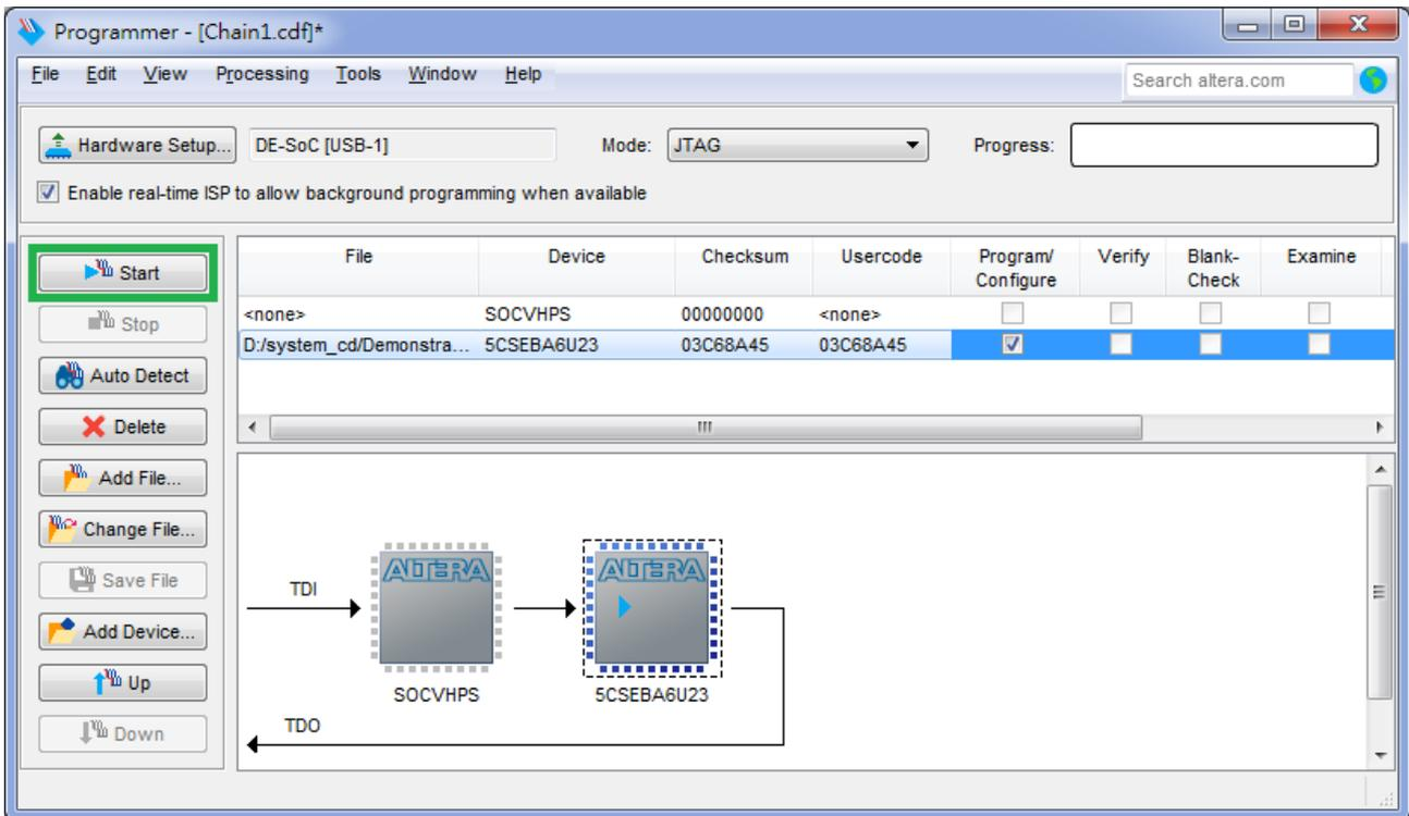
**Figure 3-10** Program.sof file into the FPGA device
