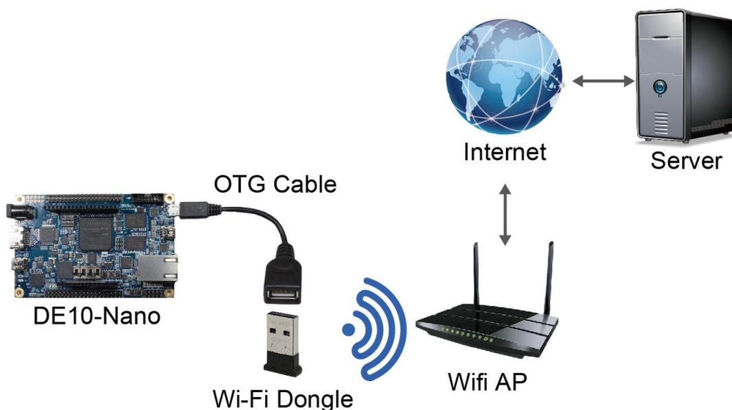
**Figure 6-9** System diagram of USB Wi-Fi dongle
