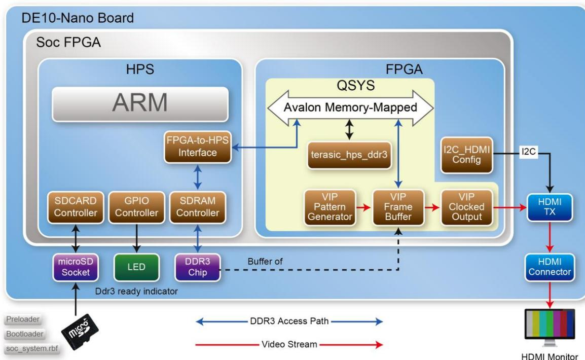
**Figure 5-9 Block Diagram of the DDR3\_VIP Demonstration**
