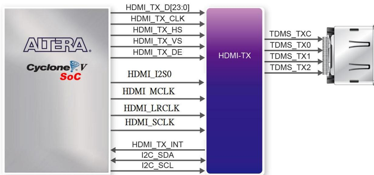
**Figure 3-24** Connections between the Cyclone V SoC FPGA and HDMI Transmitter Chip
