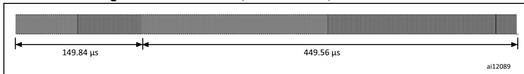
Figure 46. End of frame, low data rate, two subcarriers
